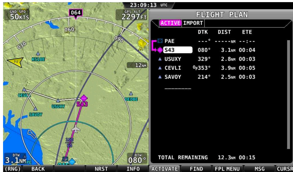
Figure 99 - Active Flight Plan: Map and Flight Plan View
