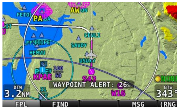
Figure 98 - Flight Plan Alert Messages
