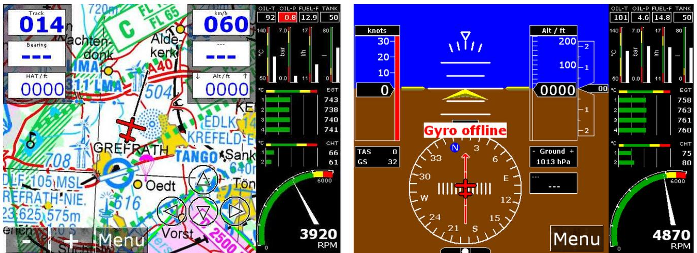
Figure 5-4-1-2, Engine Instruments on Flymap Screens
