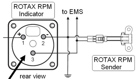
Figure 3-2-5-5, ROTAX RPM Sender
