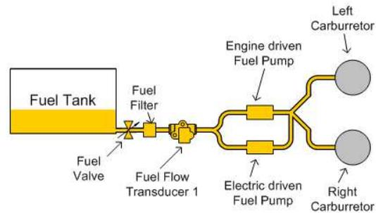
Figure 3-1-5-1, Tank Installations without Fuel Return Line
