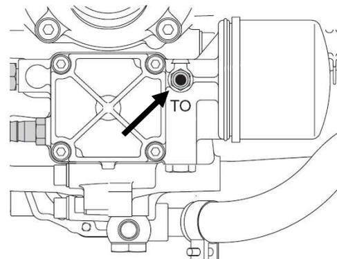
Figure 3-2-5-2, ROTAX Oil Temperature Probe
