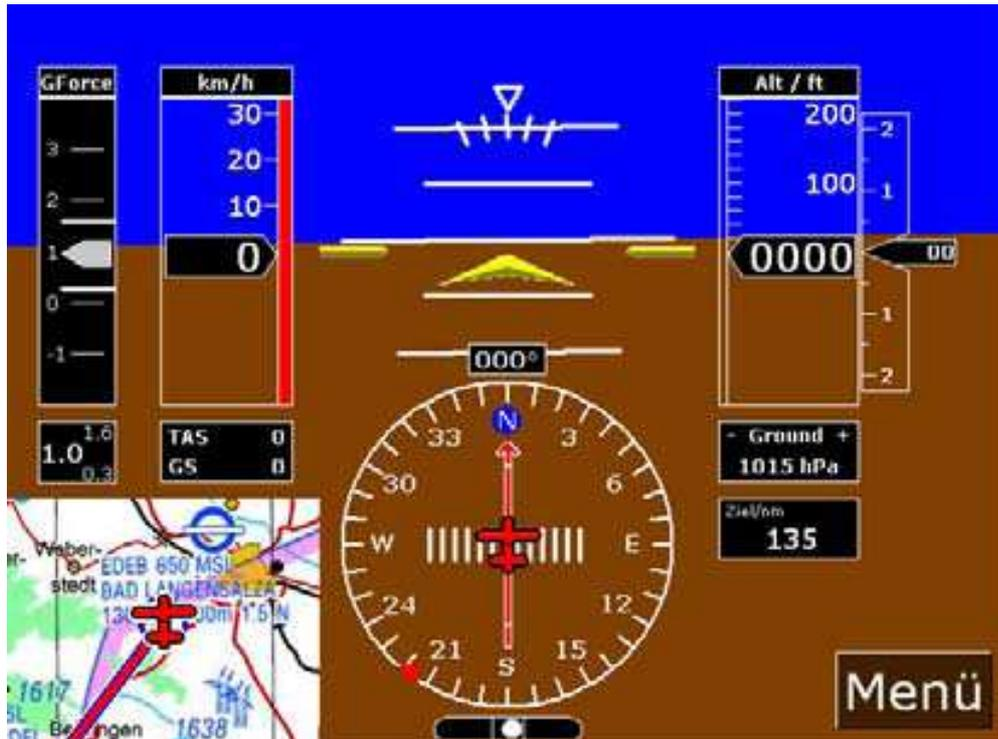
Figure 1-3-3, Primary Flight Display with Map Window
