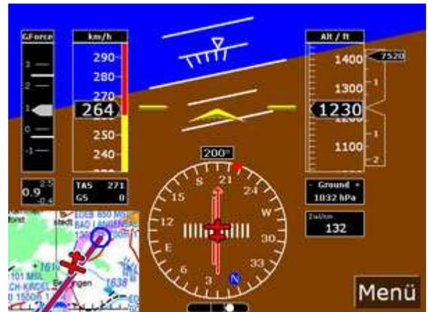
Figure 5-3-2-4, PFD with map window descending in right turn with overspeed.
