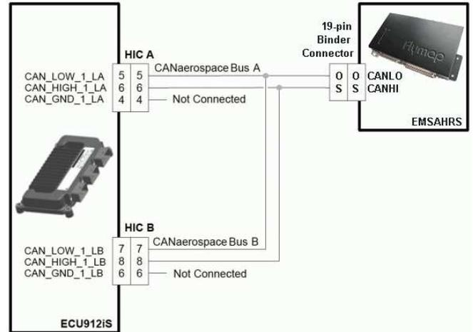
Figure 3-2-1, CANaerospace Bus Connection
