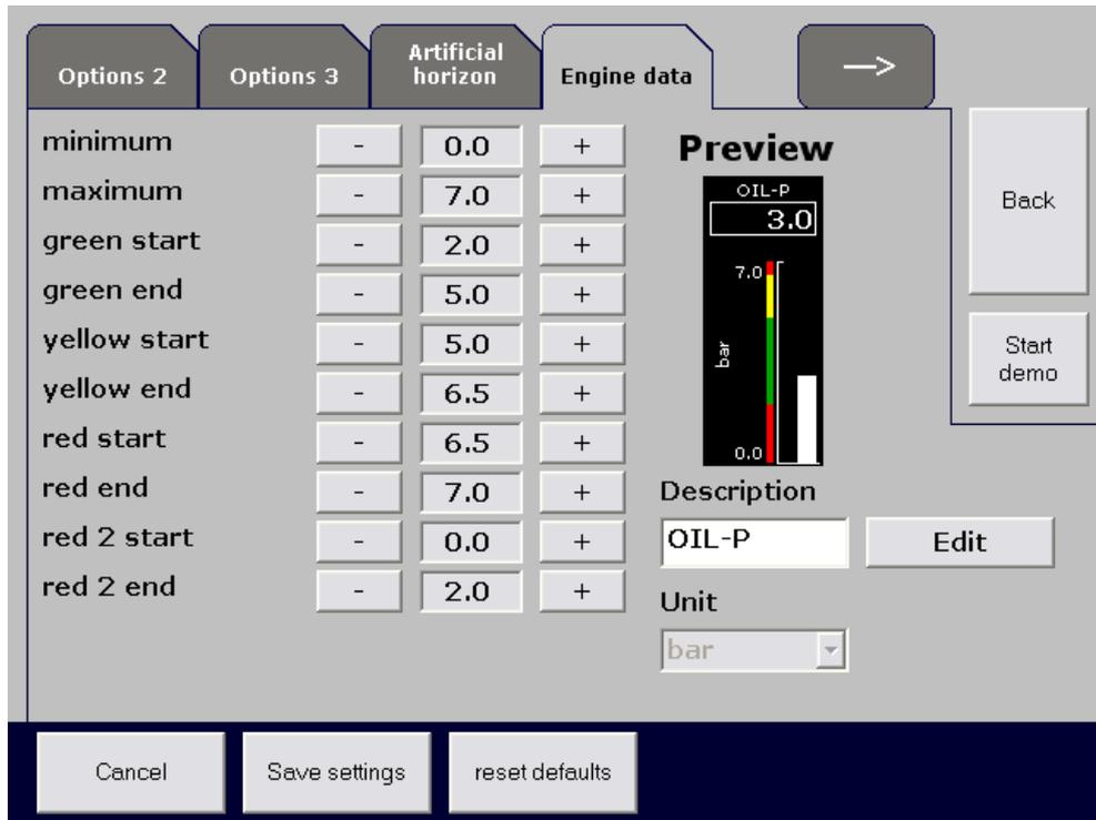
Figure 5-4-2, Instrument Configuration Page
