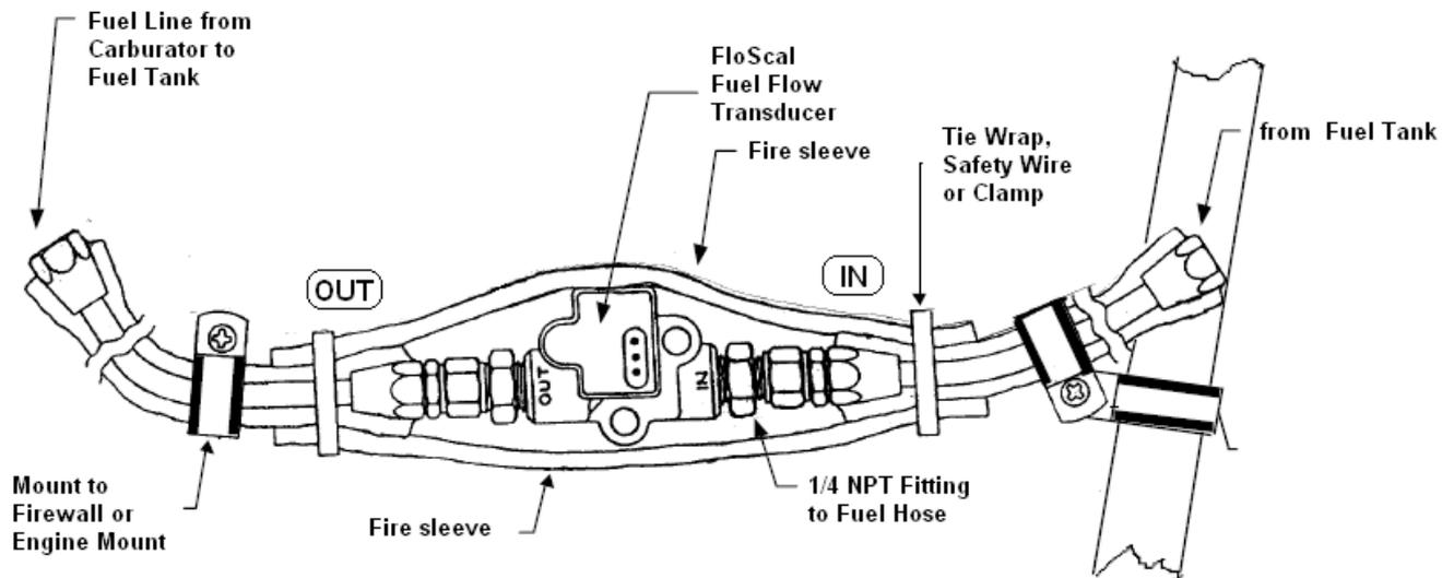
Figure 3-1-5-3, Mounting of the Fuel Flow Transducer
