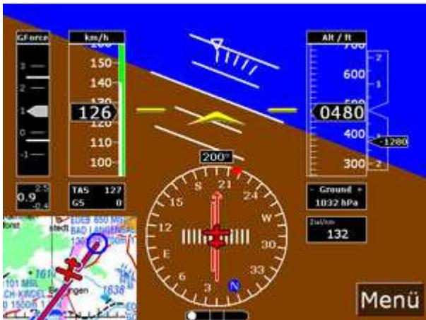
Figure 5-3-2-3 PFD with map window descending in left turn (slipping)
