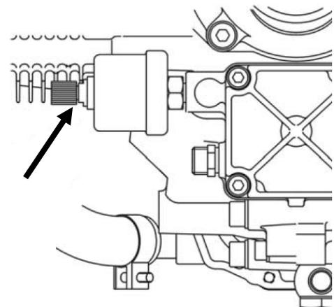
Figure 3-2-5-7, ROTAX Oil Pressure Sender
