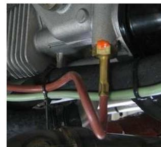
Figure 3-1-3 CHT Probe Installation
