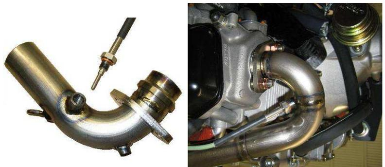
Figure 3-1-6, EGT Probe Installation
