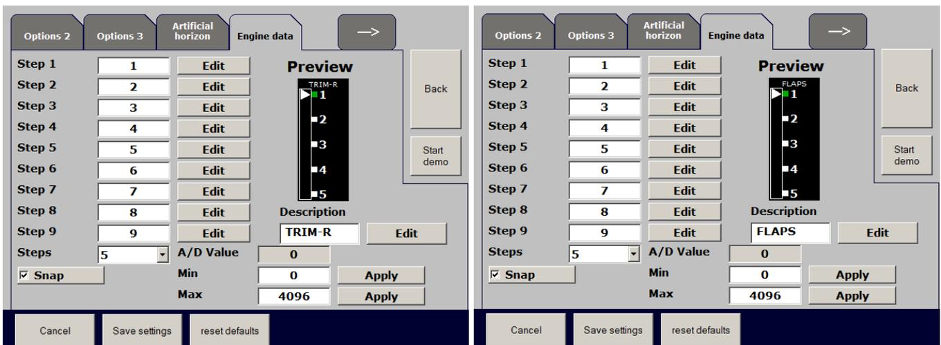
Figure 5-4-4 Trim- and Flap Position Indicator Configuration Page
