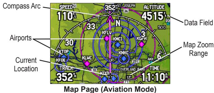
A navigation arc (Horizontal Situation Indicator, or HSI) appears by default on the Map Page. The arc works like the compass on the Panel Page, indicating the course and your deviation left/right of this course. If the route line and magenta arrow are heading straight up, you are heading directly to your destination.
