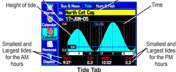
The top of the page shows the tide station and date being referenced. The chart shows a 24-hour block of time, with the time progressing from left to right. The solid vertical lines represent 4-hour increments; the dotted vertical lines represent 1-hour increments.
