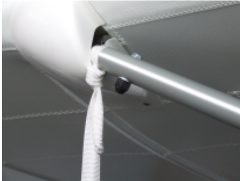
Tie down point at the upper front strut area.
