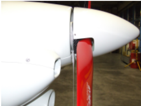
Tie down point between the engine cowling and propeller spinner.
